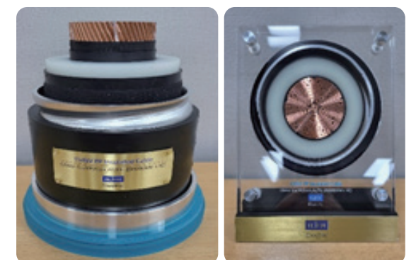
154kV CU/PP/Corr.AL/PE 2500SQMM
